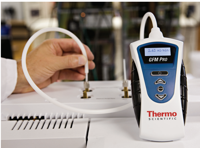
Figure 4. Probe connected to a GC gas outlet.
